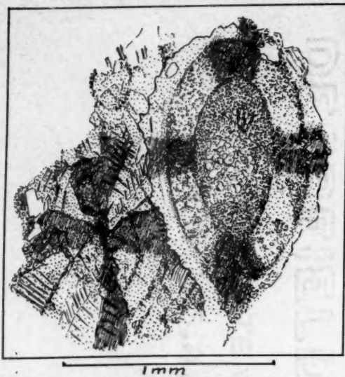
FIGURE 1. LAY. RED SPHERULITE AND SPHERULITIC MUD PELLET. Both show growth aprons beyond their original boundaries after deformation. Beekmantown (Ordovician). Paradise church 4 1/2 miles NNE. center of Hagerstown. ac section, deformation 20 per cent, spec. 357, Hagerstown quadrangle.
